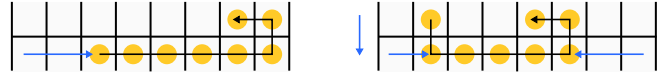
Fig. 5. Examples of flat layouts for N = 8 stitches. Left: single-fold with r = 2 , right: c-shaped with s = F , l = 1 , r = 2 and m = 5 .
